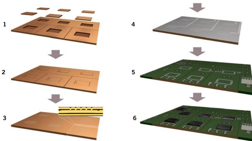
1. Cu lead frames with cavities as carriers for power Mosfets with Cu metallization
