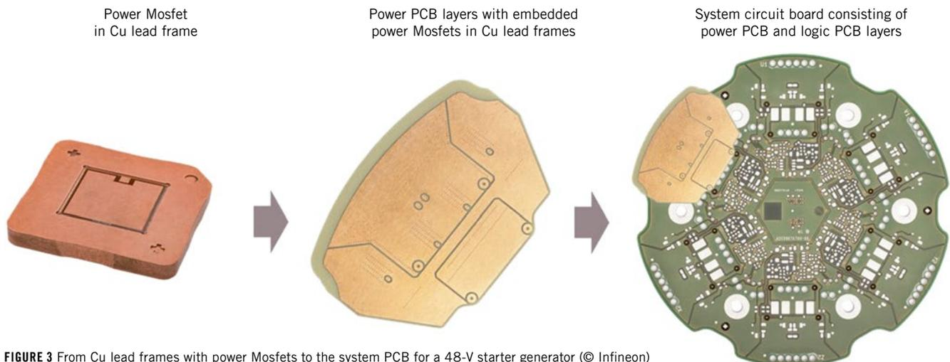
FIGURE 3 From Cu lead frames with power Mosfets to the system PCB for a 48-V starter generator (© Infineon)
