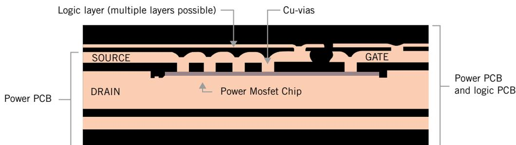
**FIGURE 1** Micrograph: chip embedding technology with power Mosfets as a system circuit board (power and logic) (© Infineon)
